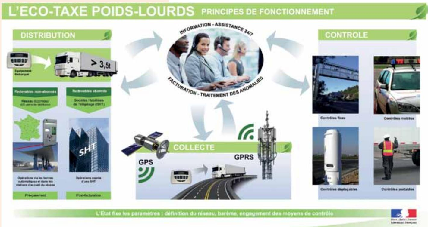
This is based on on-board equipment installed on the vehicles, which, using an advanced satellite system, enables the very accurate positioning and identification of the vehicle and ensures taxation applied only on the distance actually travelled. This on-board equipment will be technically interoperable with other tolling schemes at a national and international level.
